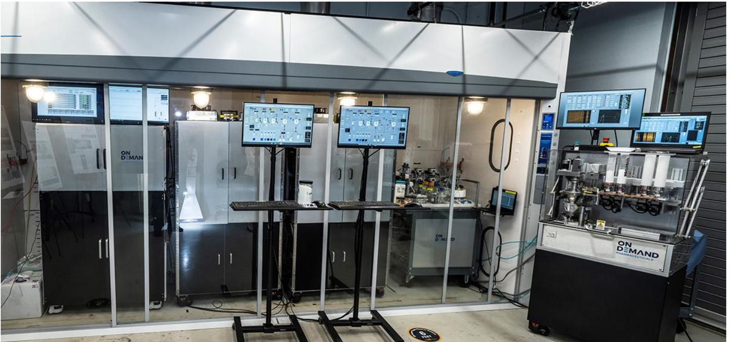
□ The automated, small-footprint, continuous manufacturing platform for the production of Ciprofloxacin developed by On Demand Pharmaceuticals as part of DARPA's Make-It programme. (Photo: On Demand Pharmaceuticals)
